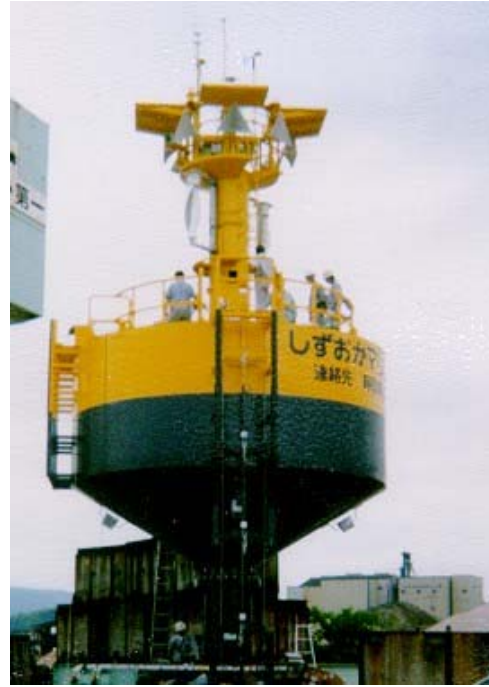
Assembling work of two WS-0,30A onto a buoy
