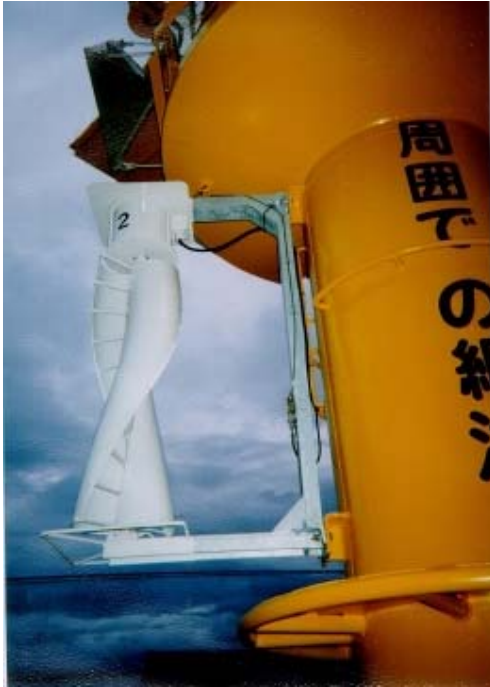
WS-0,30A with automatic lubrication system in a buoy in the Pacific Ocean
