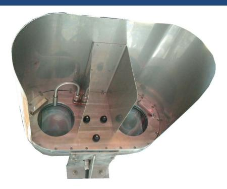
The FD-410A fog detector is a microprocessor device designed to automatically detect and execute the control functions for a fog signal, traffic signage or other devices, when visibility has decreased below a preprogrammed level.
