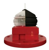
IALA Recommendation 0-113 and USCG 33 CFR 118 Approved. Lights required by the regulations shall be of sufficient candlepower as to be visible against the background lighting at a distance of at least 2,000 yards on 90 percent of the nights of the year. They are located as prescribed, with colors and arcs of visibility as specified.
